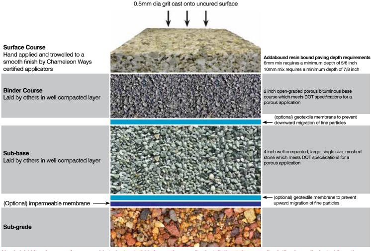
Newly laid bituminous surfaces are able to be treated 30 days or longer after installation to be sure all volatiles have dissipated from the surface. Newly placed concrete surfaces are able to be treated upon complete cure of concrete approximately 30-90 days after placement. If areas need to be installed sooner please consult with your approved Addabound installer.
